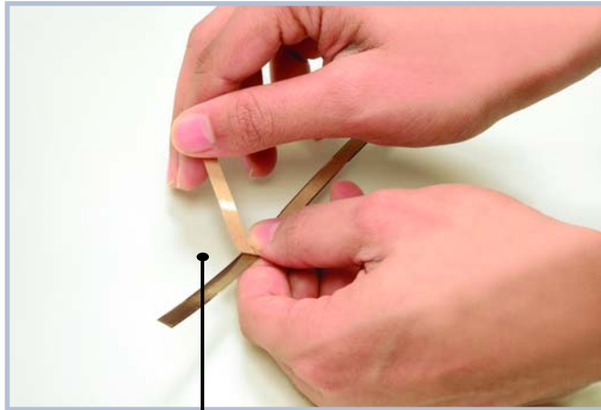
Adhesive liner peeled off about 25mm (1 inch) from the designated "LEFT END"
