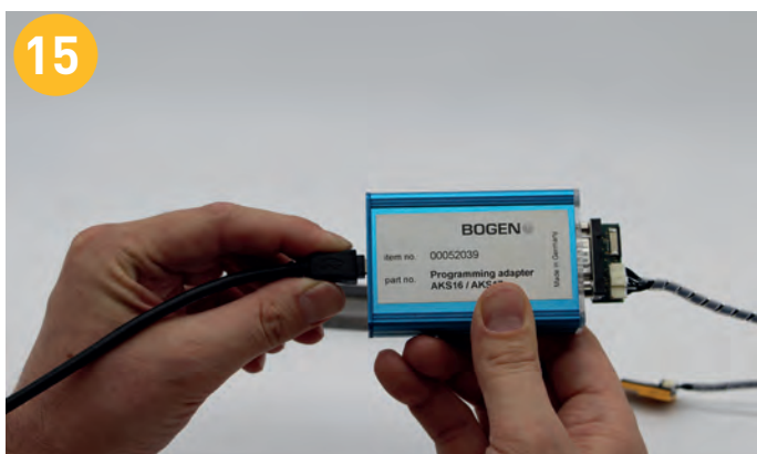
Connect the USB-cable to the calibration unit.
