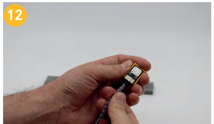
Attach the connector cable to the encoder.
