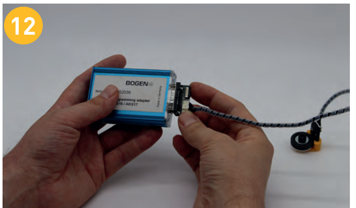
12 Connect the encoder to the calibration unit.
