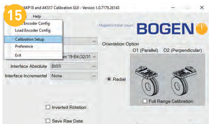
Start the calibration software and select the calibration setup.
