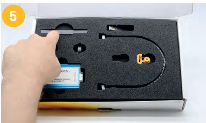
Select the linear scale and remove the double sided adhesive.
