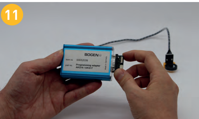
11 Mount the adapter to the calibration unit.
