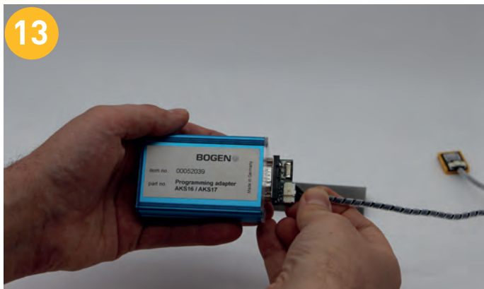
Connect the encoder to the calibration unit.
