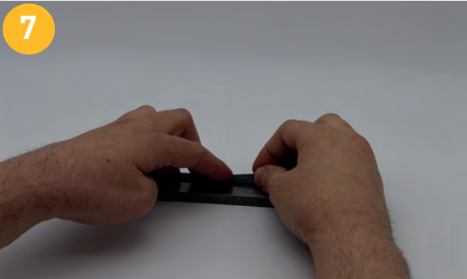
Mount the scale onto a clean and flat surface. The master and nonius tracks are labelled with arrows and the letters M & N.
