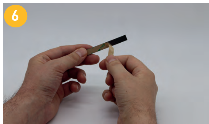
Assemble the mount and the encoder. The sensing Element is supposed to be positioned over the slot over the scale.
