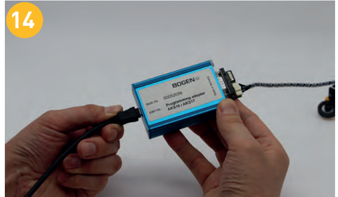
Connect the calibration unit to the USB Cable.
