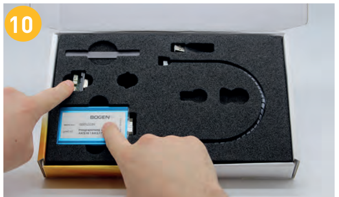
10 Select the calibration unit and the adapter.
